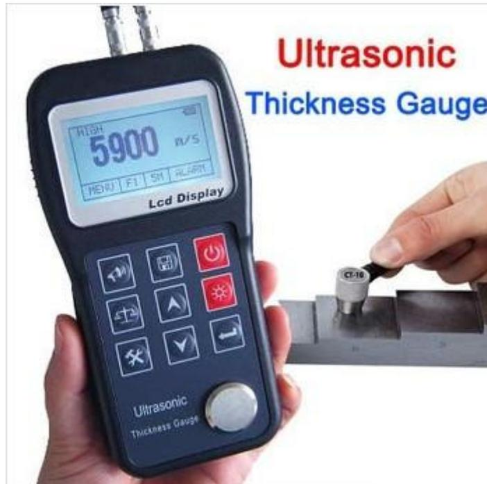
measuring with ultrasonic wave, is applicable for measuring the thickness of any material in which ultrasonic wave can be transmitted and reflected back from the other face.
