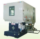
Z溫度/濕度/震動三綜合試驗系統 Z Temperature Humidity Vibration Combined Test System
