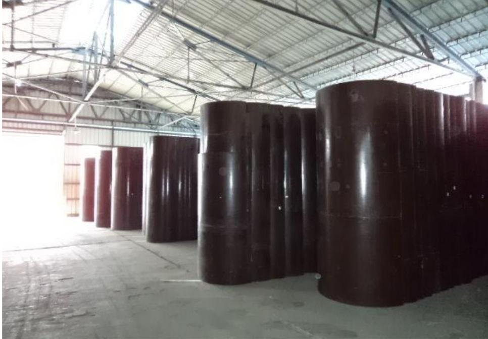
**Usage:** it's used for concrete forming of pillars/columns in buildings, such as express way bridges, and so on.
